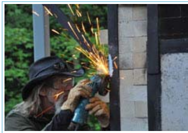
Wm. Reeder Fahnestock grinding welds on the steel frame of Watershed's new wood fired kiln, June 2010.
